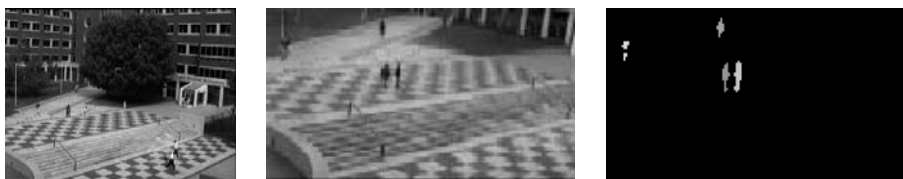
Figure 3: Typical Image from pedestrian plaza. Background mean image, input image with blob bounding boxes and blob segmentation image
