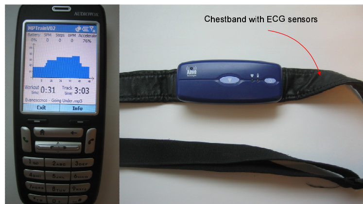
Figure 3: MPTrain's Hardware: On the left, the mobile phone (Audiovox SMT5600) and on the right, the Alivetec heart monitor and 2-axis accelerometer with Bluetooth.
