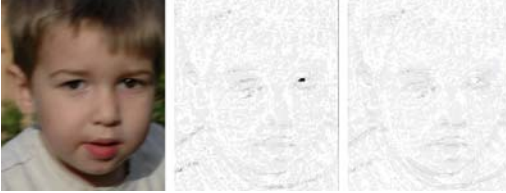
Figure 3. Original out of focus and motion blurred image, with specular highlight in the boy's left eye (left), amplified sharpness map before contrast based correction (middle), amplified sharpness map after contrast based correction (right).
