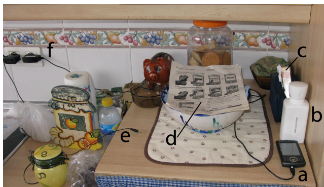
Figure 4. A typical setup of the apparatus (subject 15): (a) HTC P3300 smartphone running MoviPill; (b) MEMS pillbox containing the medication of the participant, the label on the box reported the regimen information; (c) other medications that were not part of the study; (d) instructions guide of MoviPill; (e) charger of the participant's main phone; (f) charger of the smartphone.
