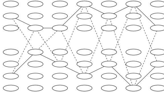
**Figure 4-17:** State trellises for a 2-chain 4-state CHMM
