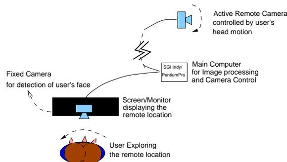
**Figure 5-3:** The virtual window: Local head positions are detected by the active tracking camera and used to control a moving camera in the remote site. The effect is that the image on the local monitor changes as if it were a window. The second image illustrates the virtual window system in use.
