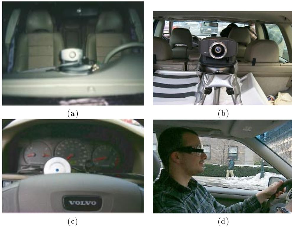
**Figure 3-8:** SmartCar sensors: (a) Front and rear wide-field-of-view cameras (b) Steering wheel sensor and driver's face camera (c) Driver's viewpoint camera
