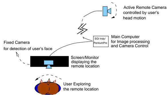
The virtual window: Local head positions are detected by the active tracking camera and used to control a moving camera in the remote site. The effect is that the image on the local monitor changes as if it were a window. The second image illustrates the virtual window system in use.
