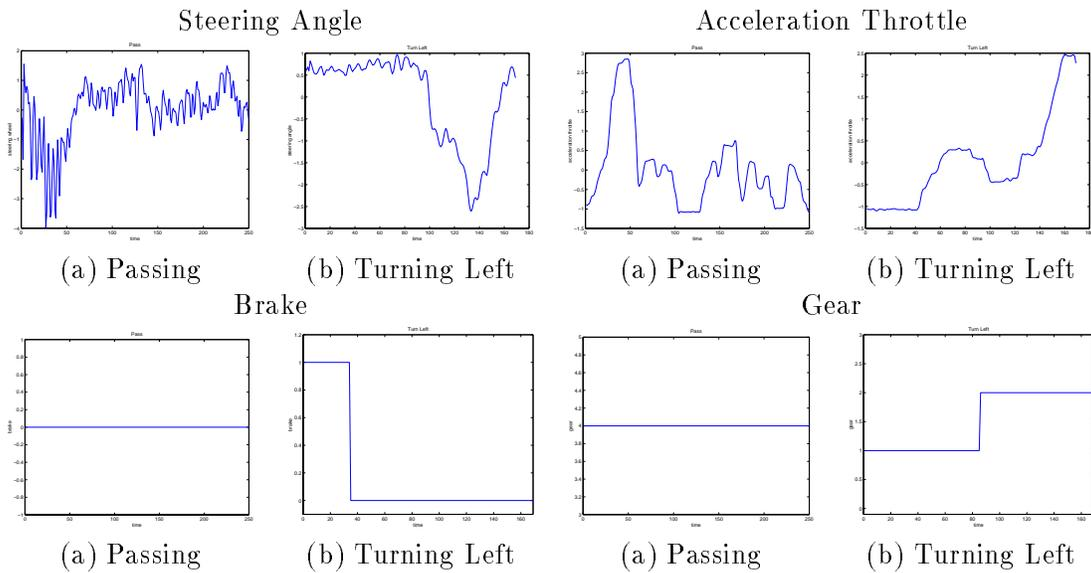
Typical car signals for passing and turning left maneuvers
