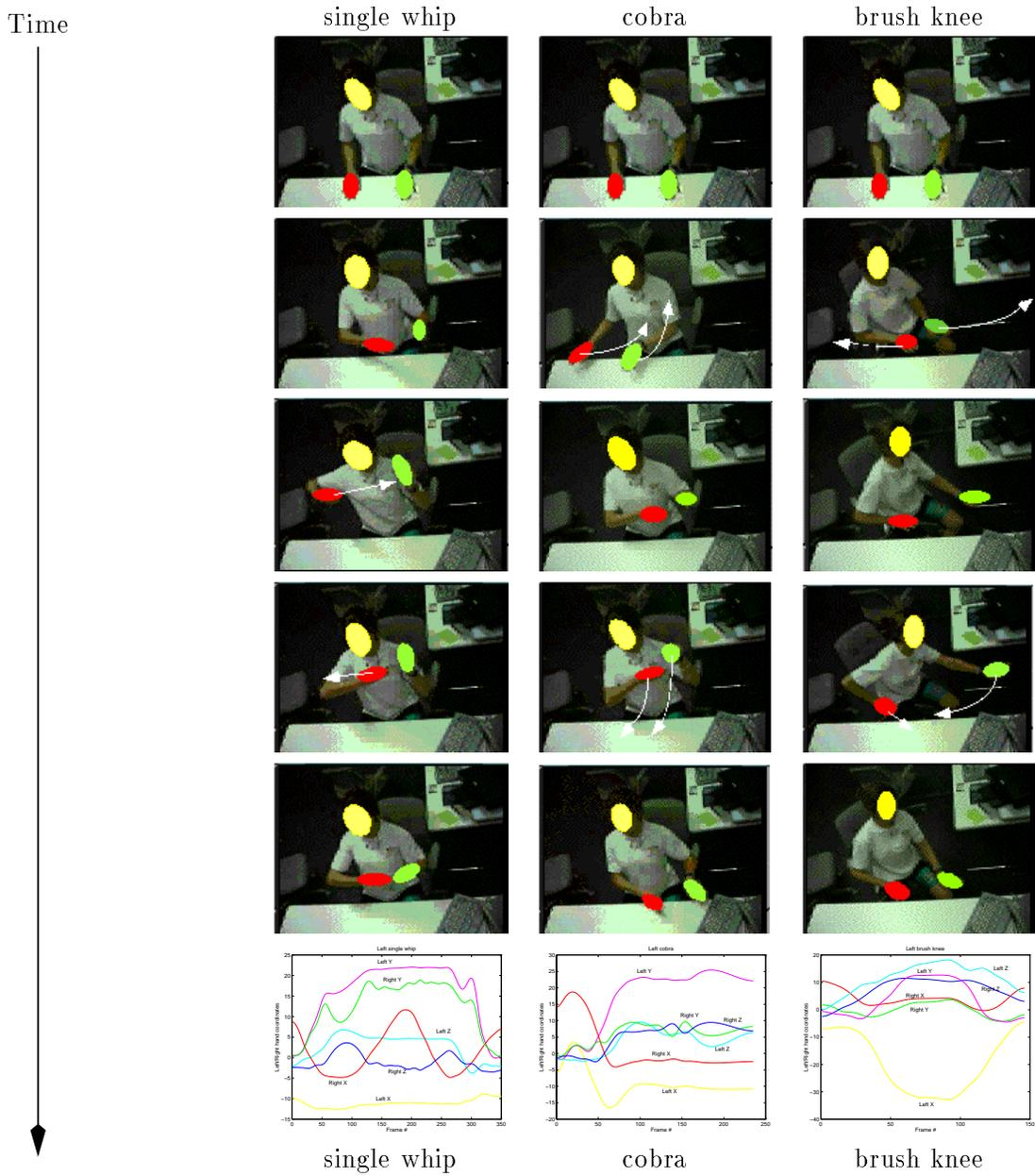
**Figure 5-8:** Hand tracking of three Tai-Chi gestures: selected frames overlaid with hand blobs from vision. The bottom-most graph shows the evolution of the feature vector over time
