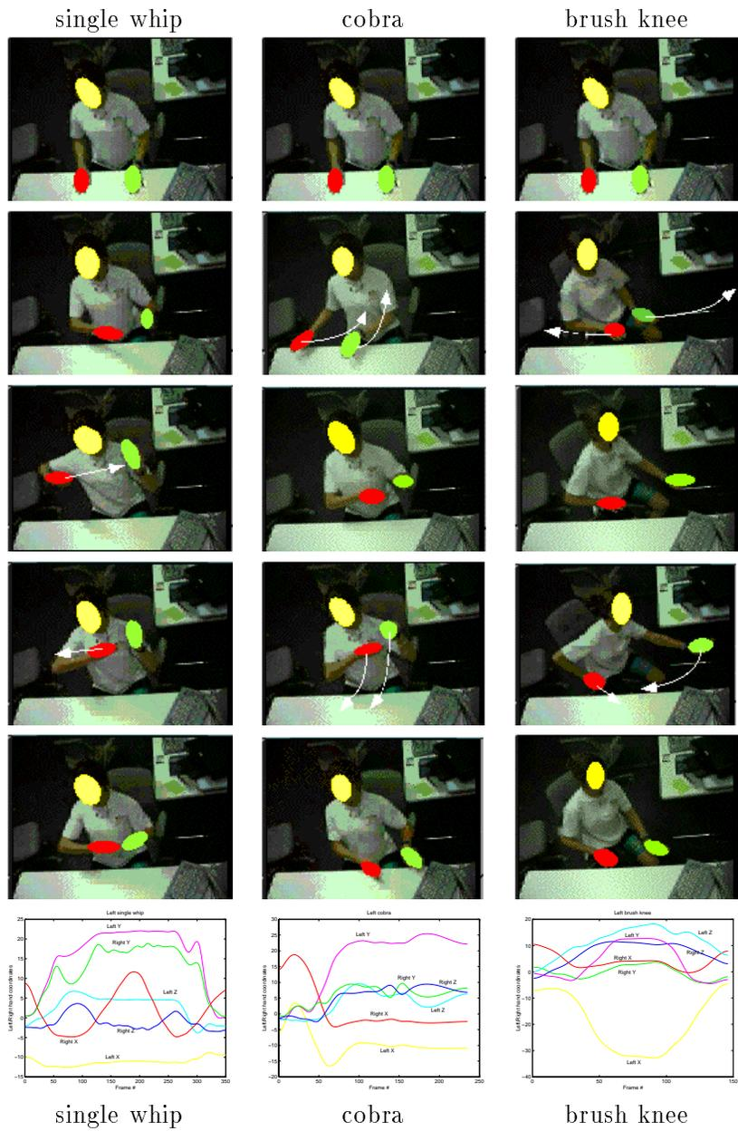
Hand tracking of three Tai-Chi gestures: selected frames overlaid with hand blobs from vision. The bottom-most graph shows the evolution of the feature vector over time
