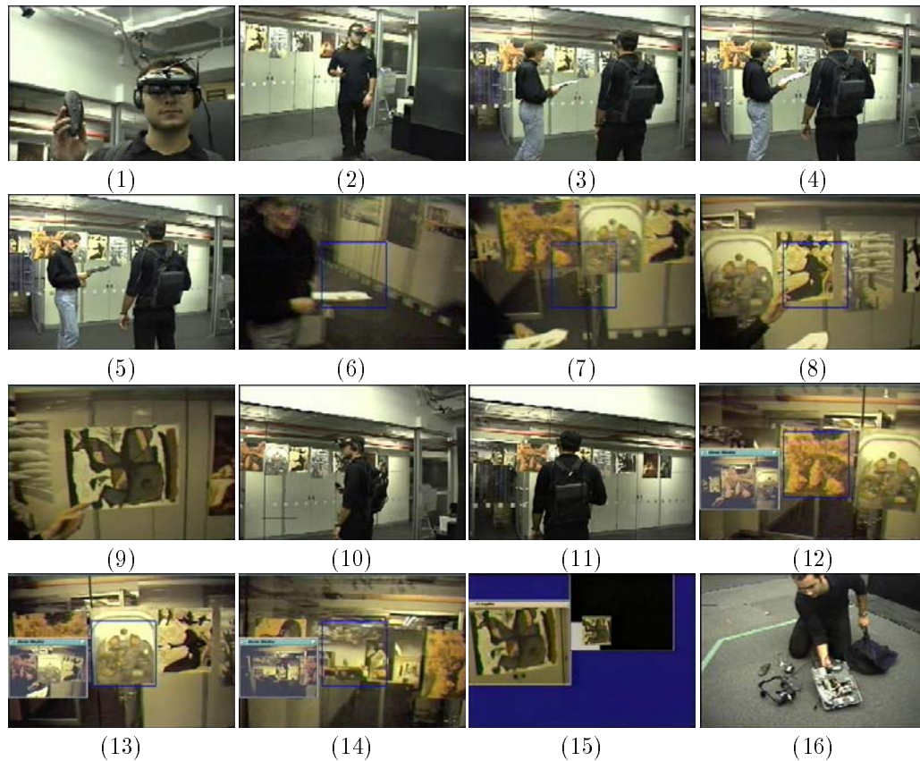
Figure 1: Training the wearable computer to act as a museum guide. (1) The user with the heads-up display and a 3-button mouse to control the system. (2) The user near several paintings in a gallery. (3-5) The guide enters the scene and points to a painting while describing it. (6-7) The guide and the scene from the user's (wearable camera) field of view. (8) The guide describes a work and points to the painting while the user records the A/V. The user clicks to associate the A/V with the image of the painting at the end of that description. (9) Another work is described, recorded and associated to the painting's image. (10-14) The user walks around the space and looks at the paintings which automatically trigger a small animation on the left window. This shows the guide explaining the works appropriately with audio and his hand gesturing over the painting. (15) The object recognition engine, demonstrating robustness in recognition to changes in pose, lighting, view angle and translation. (16) The user removing the wearable system. Note, here the visor being used is a Virtual I/O prototype, we are currently using the much small MicroOptical display shown in the Hardware section.
