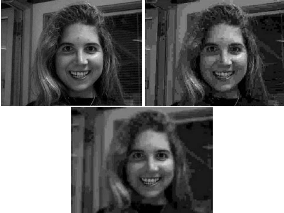
Figure 11. Preferential coding: the first image is the JPEG flat encoded image (File size of 14.1Kb); the second is a very low resolution JPEG encoded image using flat coding (File size of 7.1Kb); the third one is a preferential coding encoded image with high resolution JPEG for the eyes and mouth but very low resolution JPEG coding for the face and background (File size of 7.1Kb).
