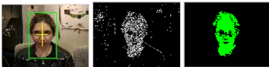
Figure 3. Face detection, per-pixel probability image computation and face blob growing
